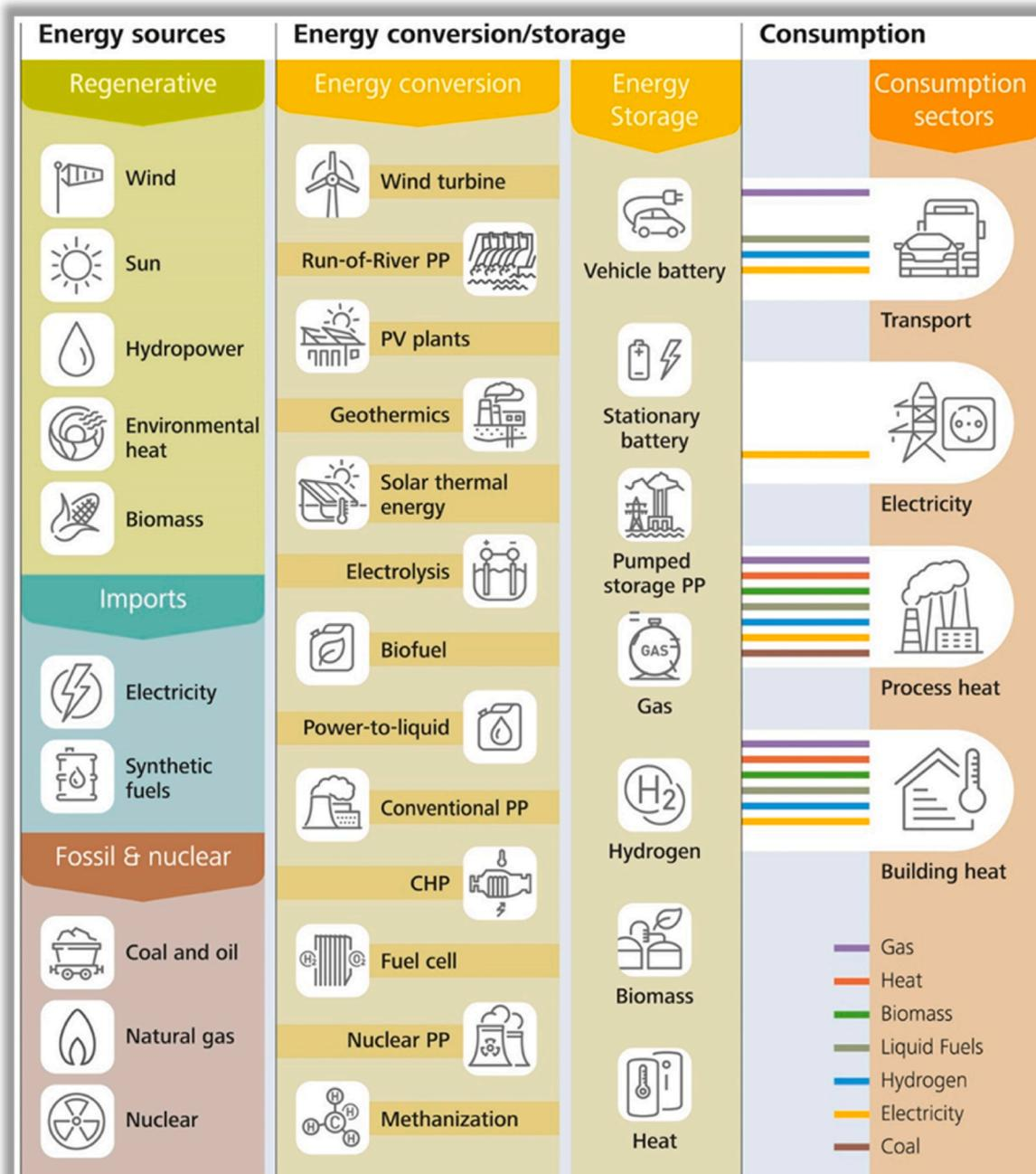
Fig. 1. Schematic overview of basic technologies considered in REMod, own illustration.
