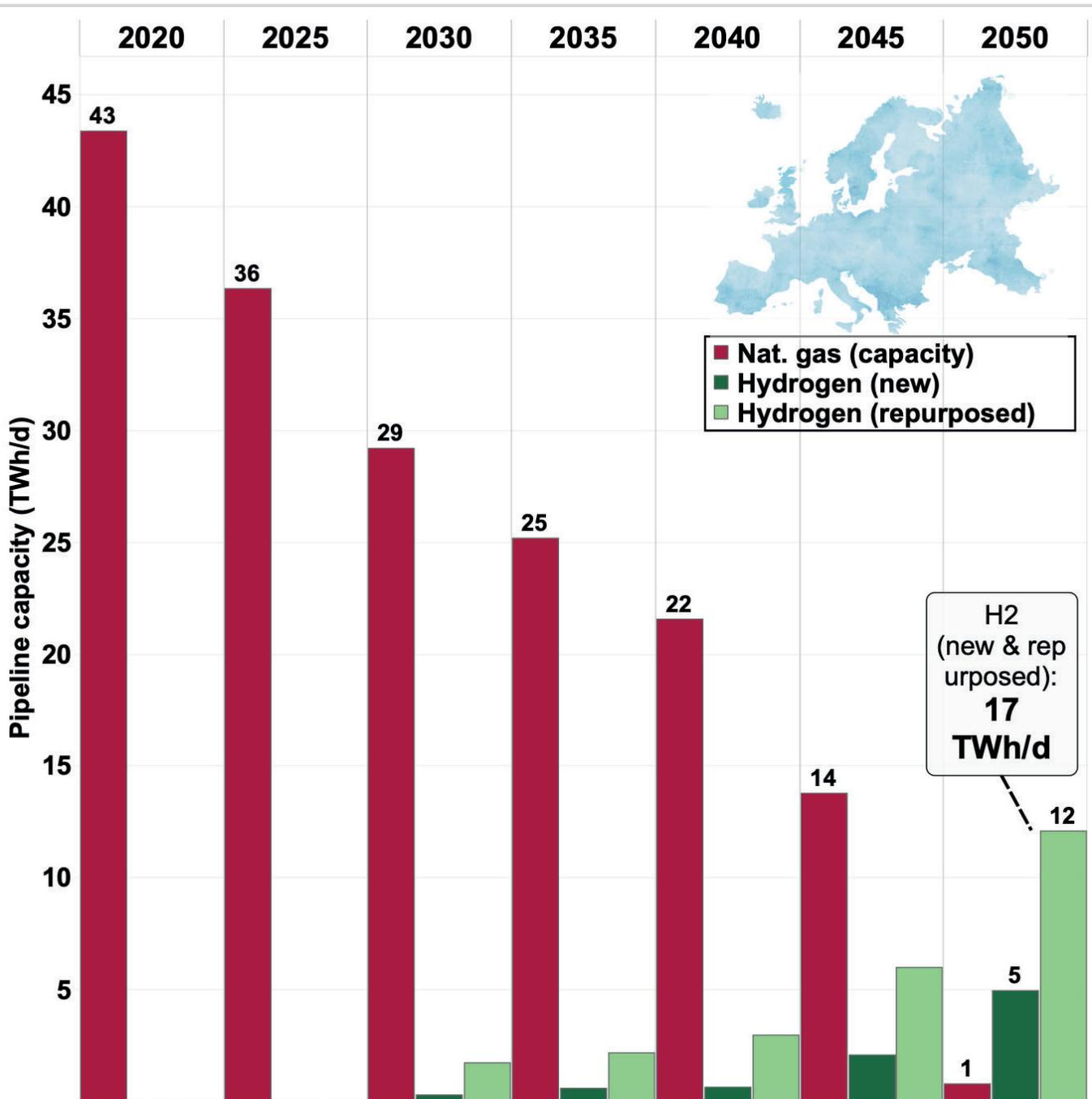
Figure 11: European pipeline transmission capacity for natural gas and hydrogen (2020-2050).
