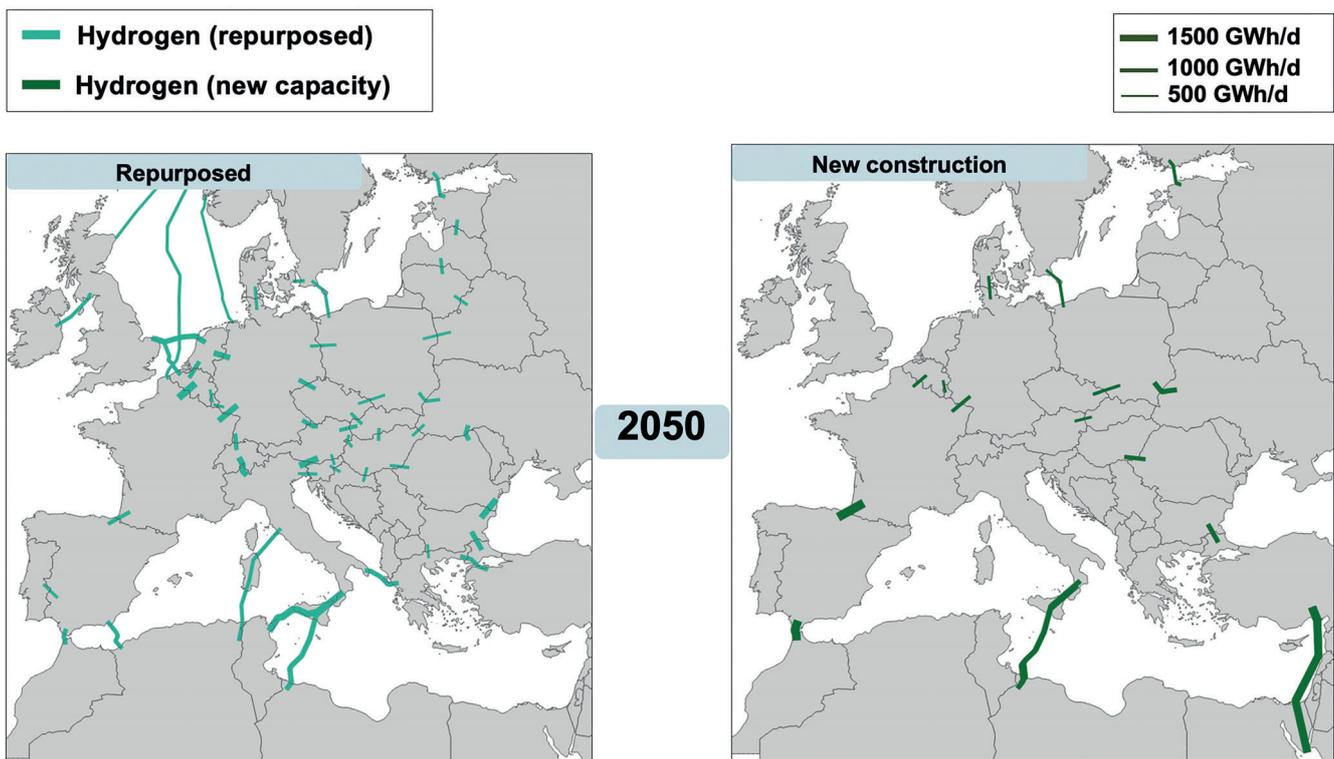
Figure 12: Hydrogen (new and repurposed) pipeline transport capacity (2020-2050).
