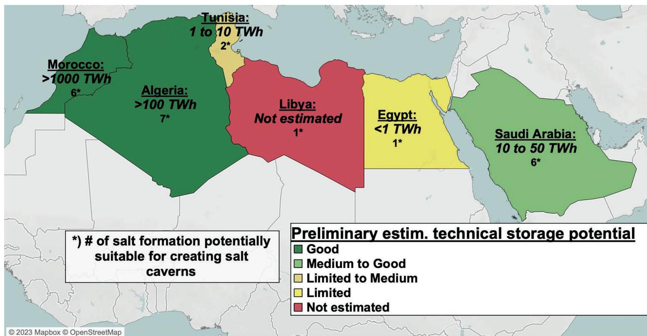
Figure 20: Storage potential and numbers of salt formations potentially suitable for creating salt caverns. Sources: Caglayan et al. (2020); Horvath et al. (2018); Jannel and Torquet (2022); Weber (2018).
